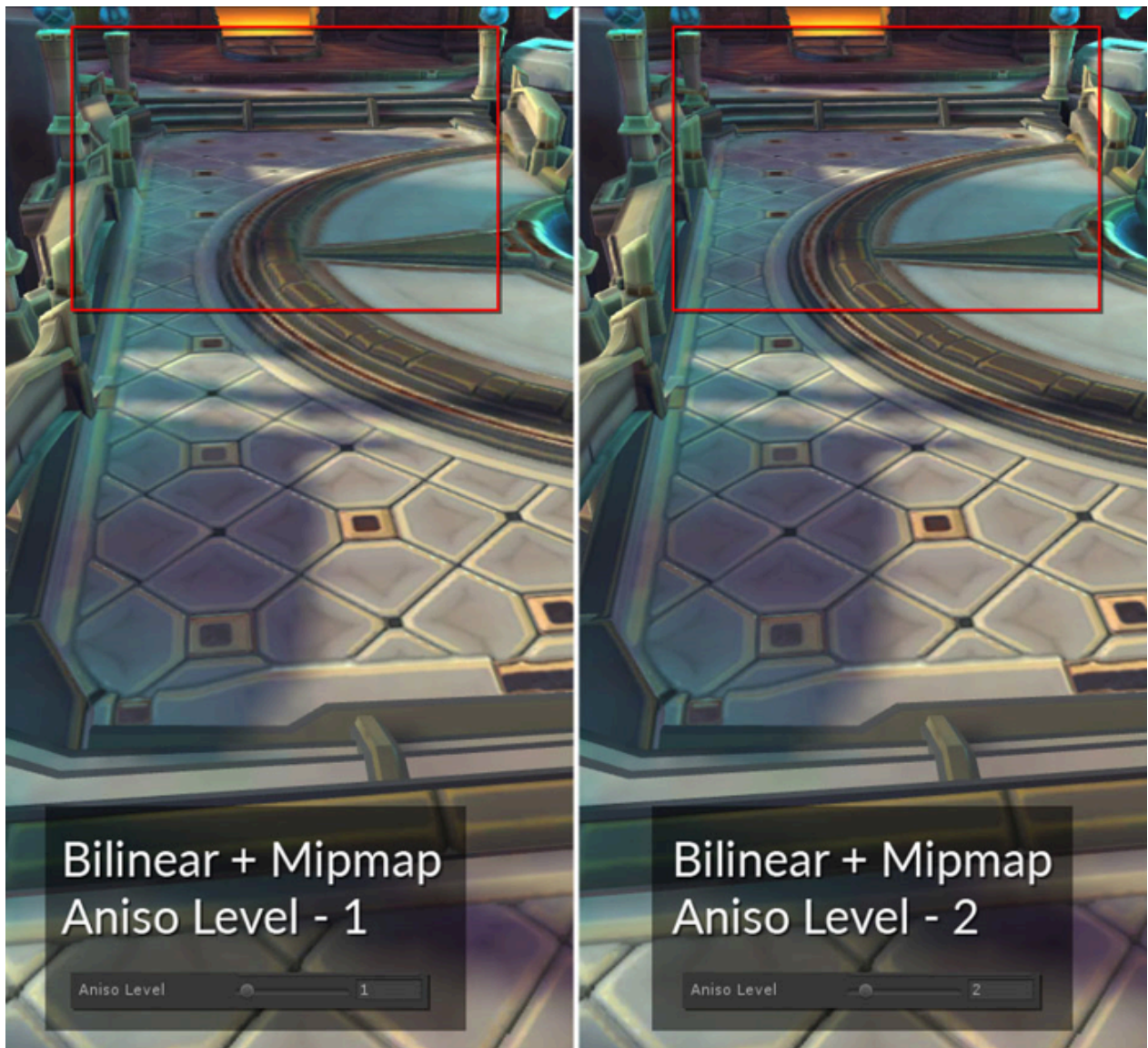
Figure 3-3: Anisotropic filtering
